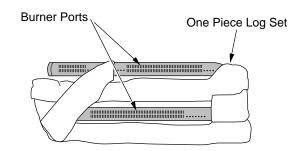
Figure 28 - Installing One-Piece Log set (Top View)
